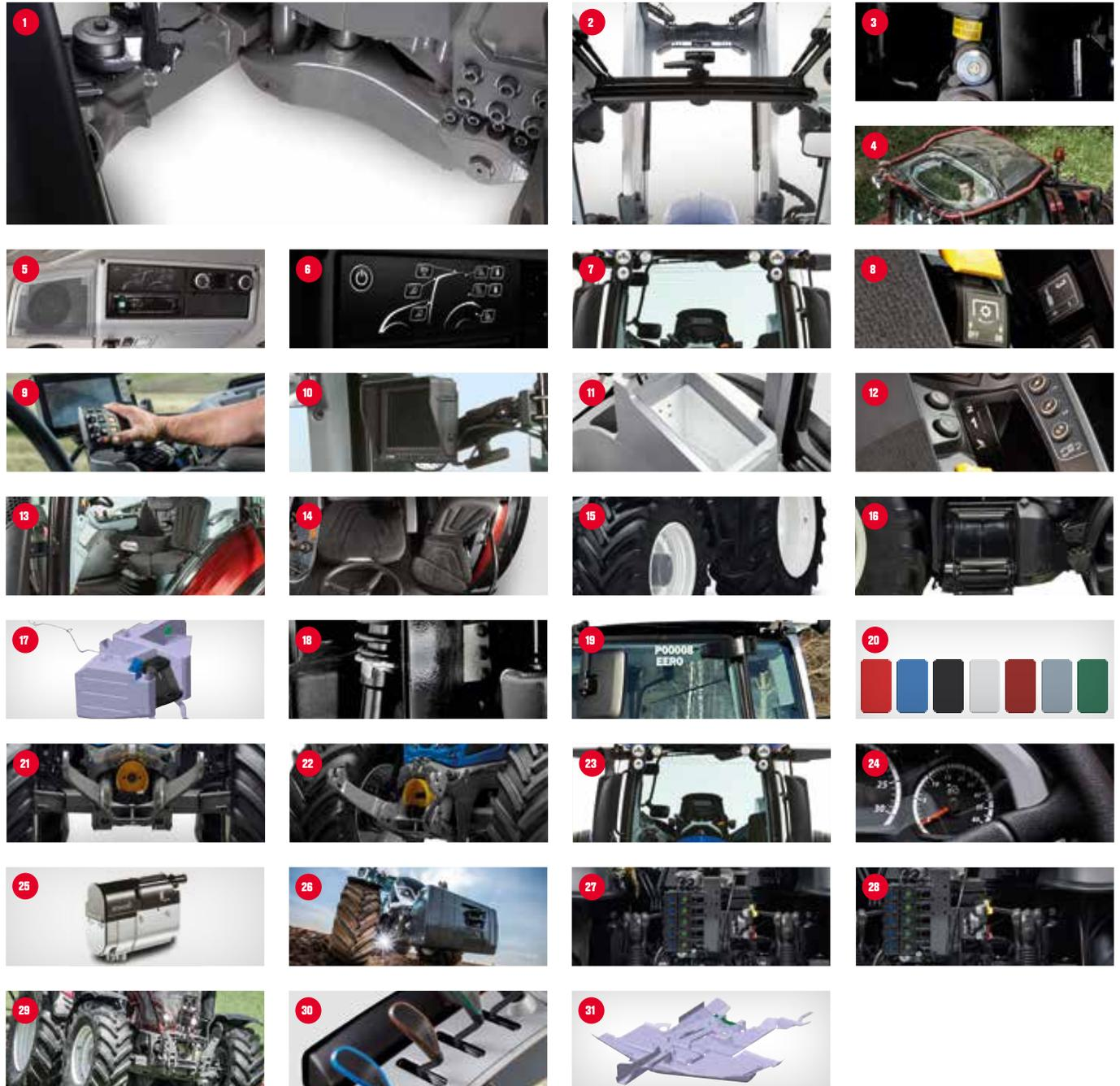
1. **Hydraulic front axle suspension** / With 100 mm travel, superb oscillation and a 7,5 ton load capacity, the hydro pneumatic suspension offers excellent ride comfort for all tasks.
