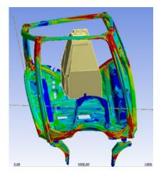
The role of simulators is growing all the time. In this picture, a simulator is being used to test the torque rigidity of a cab frame.
