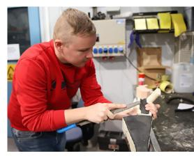
Industrial Designer Henri Hokkanen works on a plastic model of an armrest. A lot of plastic, wood and 3D-printed components are used in the design studio to make full-size mock-up models of future tractors and cabs.
