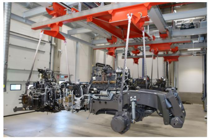
In the new paint shop, tractor chassis hang by chains from a conveyor. This allows the painting robots to move around them without hindrance. In addition, the new paint shop is more flexible, more spacious and enables the production of even bigger tractors.
