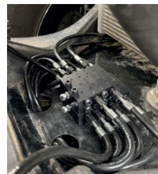
S series front axle and front linkage central lubrication system.
