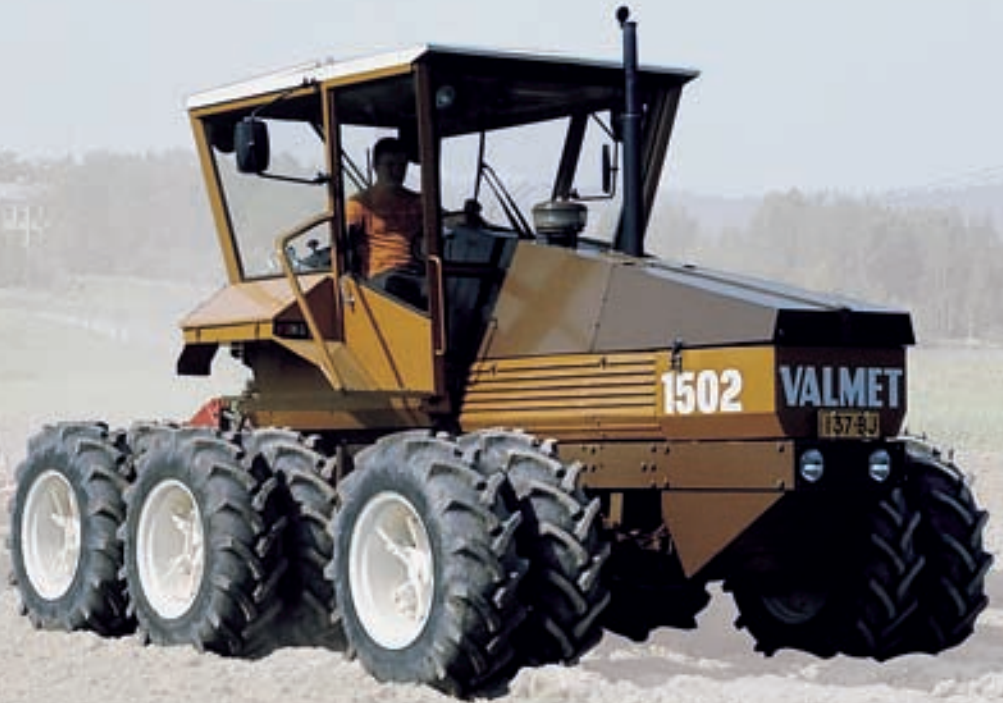
The Valmet 1502 was an impressive sight. The tractor offered improved pulling capabilities and steering properties with a propelled front axle. Since appropriate agricultural tyres could not be sourced, the tractor used 13.6-24 double wheels.
