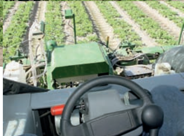
The automatic hoe makes considerable demands on a tractor's hydraulic and electrical services.
