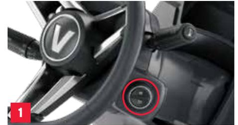
1. Use the wheel encoder and two buttons to navigate screen.
