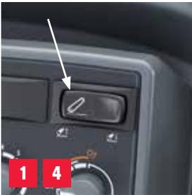
1. Press the symbol side of the lifting/lowering switch to fully raise the linkage.
