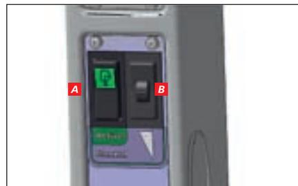
***The AutoComfort control panel is located in the right-side B-pillar in the cab. When the switch is in the centre position the damping is automatic. When it is in the lower position the system is manual and the degree of damping can be adjusted by the knob.***
