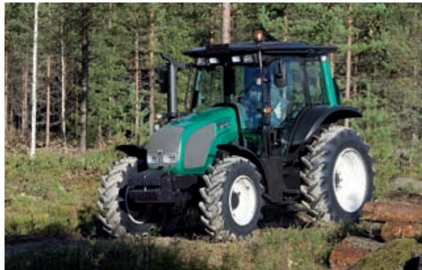
*The N Series can also be specified with a forest cab, a rear gas pedal and a protected fuel tank, making it ideal for forest use.*
