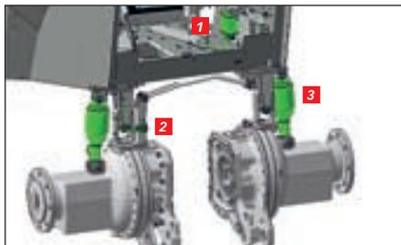
***Valtra's AutoComfort cab suspension system consists of an electronic control unit (1), a position sensor (2) and a combination air spring/CDC shock absorber (3). CDC stands for Continuous Damping Control.***
