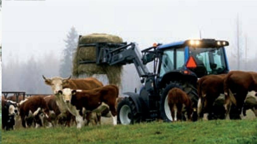
*The new N Series models are at their best in front-loader work. Visibility is excellent, the turbine clutch is precise, and the tractor is extremely well balanced when working with bales, for example, thanks to its light nose.*
