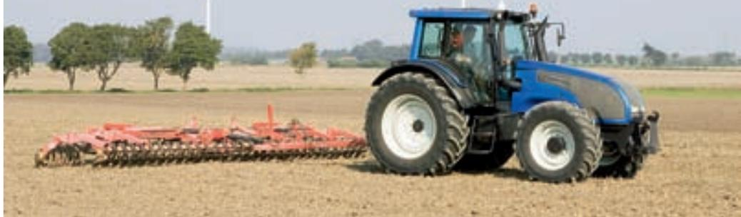
***Cab suspension on tractors has become increasingly popular, but so far all cab suspension systems have been "passive", meaning that the spring and dampening settings have been made on the basis of specific design criteria. The end result is always a compromise. Cab suspension that is good on the road may not be the best off the road.***
