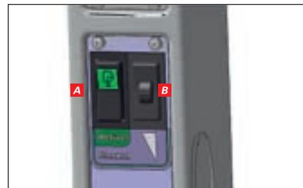
***The AutoComfort control panel is located in the right-side B-pillar in the cab. When the switch is in the centre position the damping is automatic. When it is in the lower position the system is manual and the degree of damping can be adjusted by the knob.***
