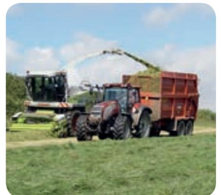
*The equipment fleet includes several 12 and 14 tonnes trailers with air brakes for safety on Dorset's rolling hills. Tractors are also equipped with exhaust brakes which have cut maintenance noticeably.*
