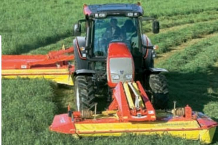
*Mowing with the new Valtra LHLINK front linkage is easier than ever. The range of adjustments eradicates underlap and overlap and offers a high quality of work.*
