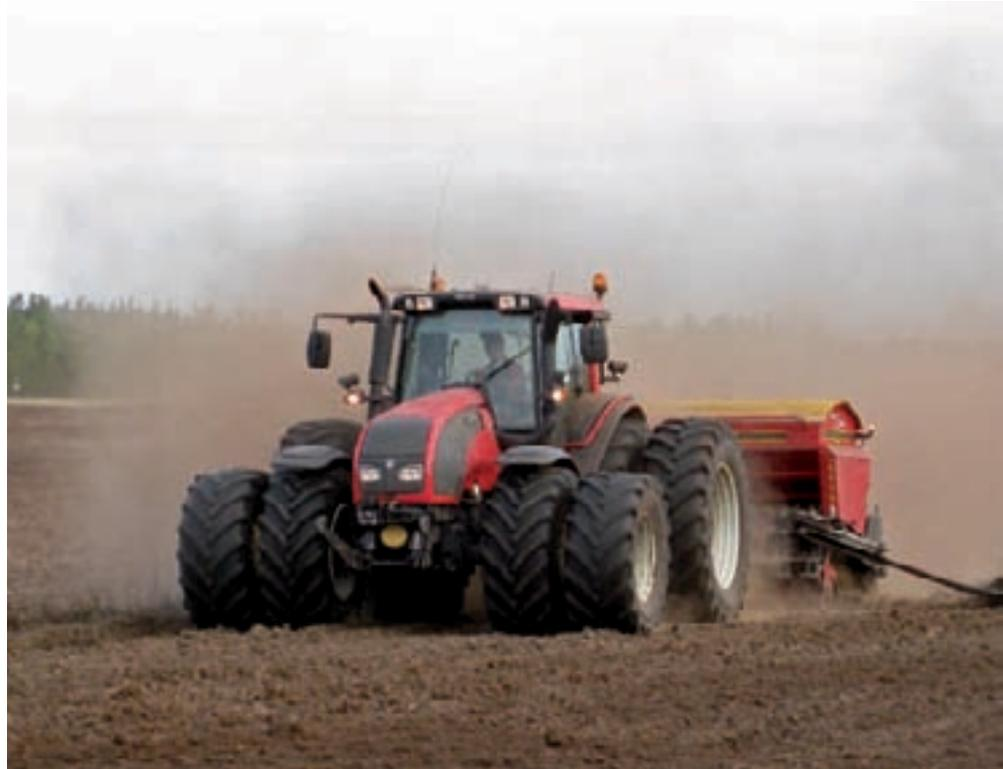
*The test tractors were used to carry out a wide range of agricultural and other contracting tasks in conditions ranging from -25°C to +30°C.*
