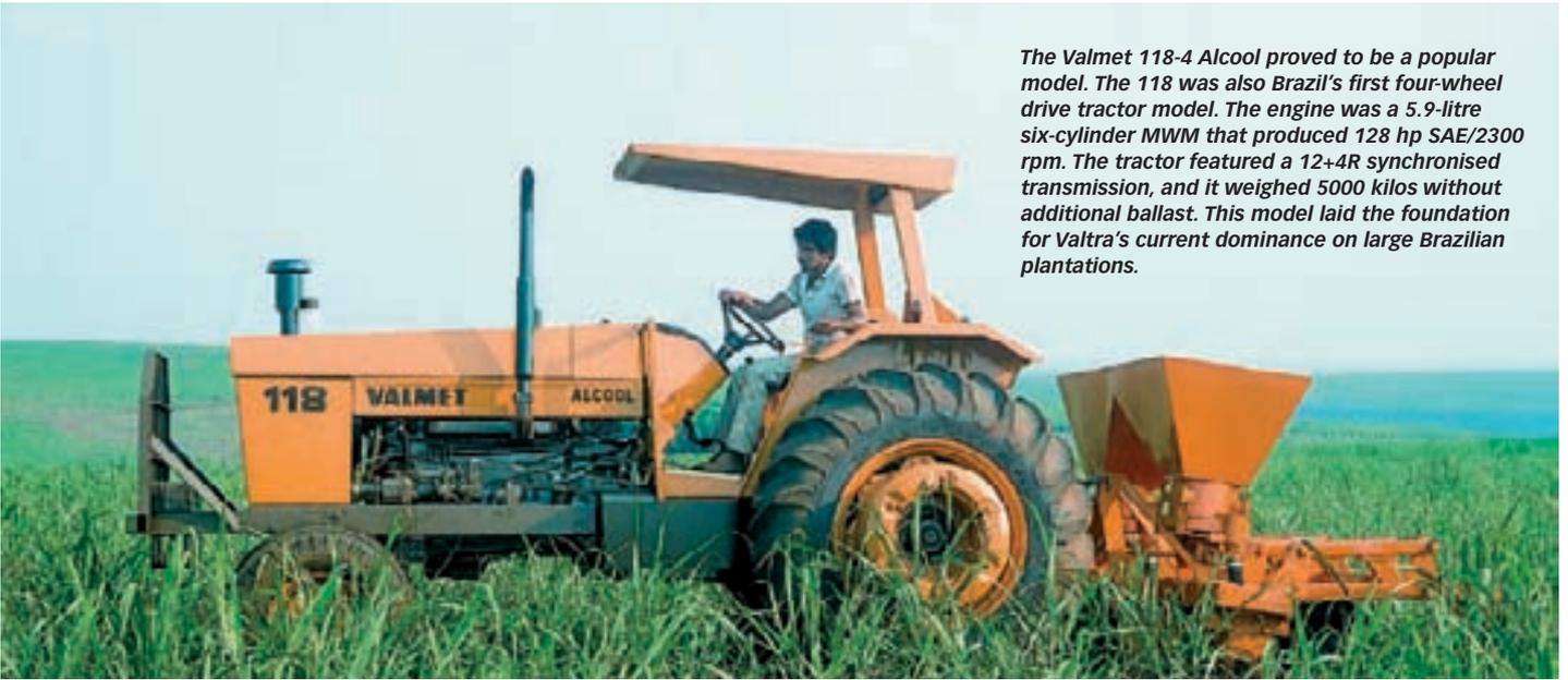
*The Valmet 118-4 Alcool proved to be a popular model. The 118 was also Brazil's first four-wheel drive tractor model. The engine was a 5.9-litre six-cylinder MWM that produced 128 hp SAE/2300 rpm. The tractor featured a 12+4R synchronised transmission, and it weighed 5000 kilos without additional ballast. This model laid the foundation for Valtra's current dominance on large Brazilian plantations.*
