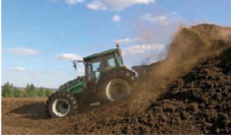
*Tractors also have to be versatile and agile for working on peat bogs. Here a Valtra N tractor is stacking peat for storage. This model offers excellent ground clearance, good protection and filtering, and the benefits of the TwinTrac reverse-drive system.*
