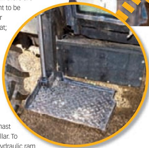
**The lift may be locked with a pin at halfway and used as a conventional step.**
