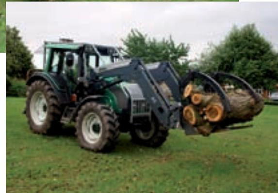
**The Valtra loader and log grab is a quick efficient way of handling large and small timber.**
