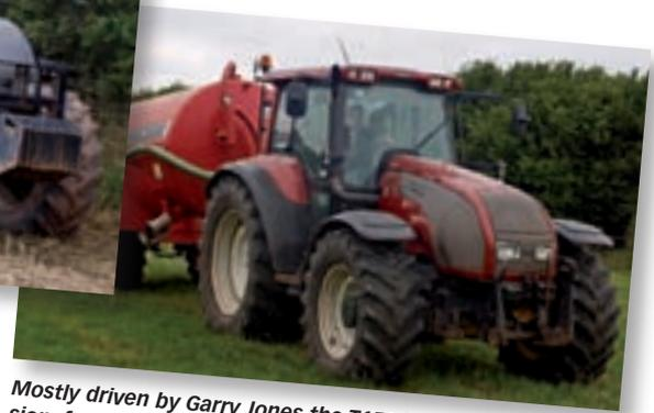
*Mostly driven by Garry Jones the T150 has a 50 kph transmission, front suspension and air brakes. Duties include heavy cultivations and road work, often with a heavy slurry tanker.*
