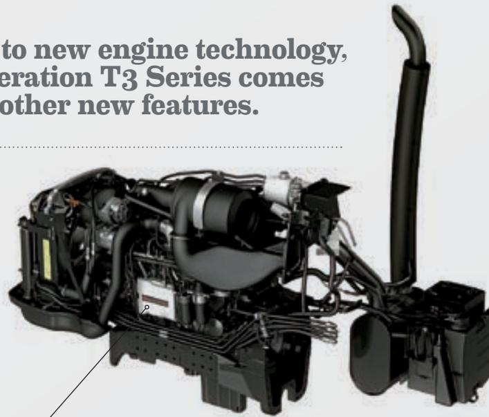
SCR technology has been used for years in S Series tractors and heavy vehicles. The onboard electronics operate the system, and all the driver has to do is fill the AdBlue tank in the same way as the fuel tank or windshield wiper fluid reservoir. SCR technology reduces fuel consumption by 5 to 10 percent and prolongs engine life.
