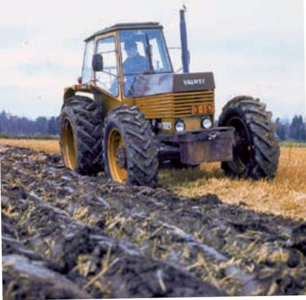
The Valmet 702S-4 was a really handy tractor with excellent traction. The tractor weighed 4040 kilos and its wheel-base was relatively long at 245 centimetres. The belly was smooth and the ground clearance higher than today's tractors in the same power class.
