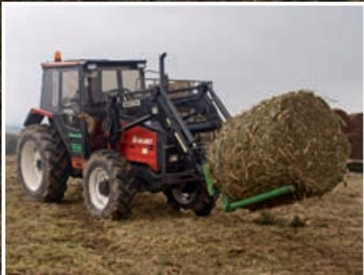
Bales of gorse weigh in at around 500 kg and are easily handled with a front loader.
