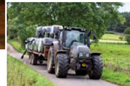
Both T Series tractors feature 50 kph transmissions, air brakes and front suspension.
