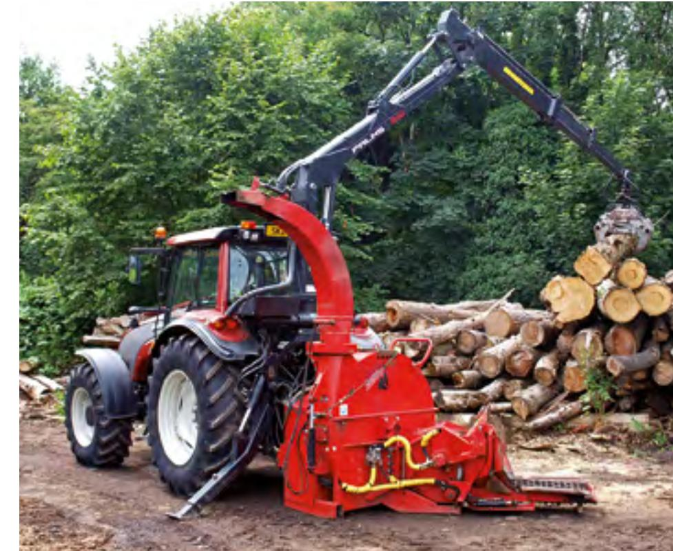
The Valtra T170 is used for chipping and in conjunction with a timber trailer for extraction, its clean underbelly and front suspension making it ideal for forestry and road operations.
