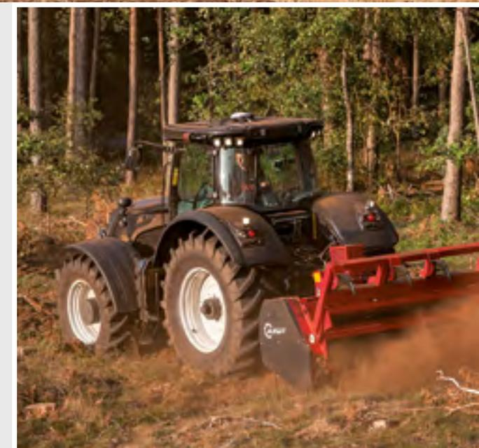
The most powerful model in the S Series produces up to 400 horsepower and 1,600 Nm of torque with boost. The engine has twin turbos and an electronically adjustable wastegate.
