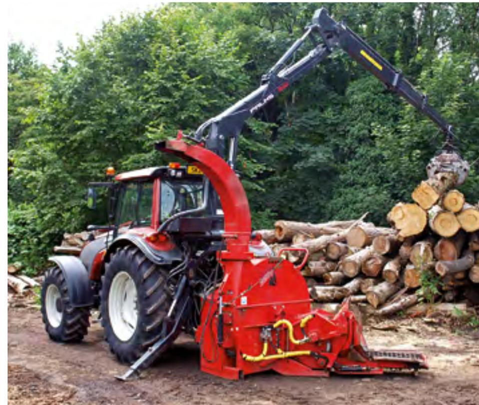
The Valtra T170 is used for chipping and in conjunction with a timber trailer for extraction, its clean underbelly and front suspension making it ideal for forestry and road operations.
