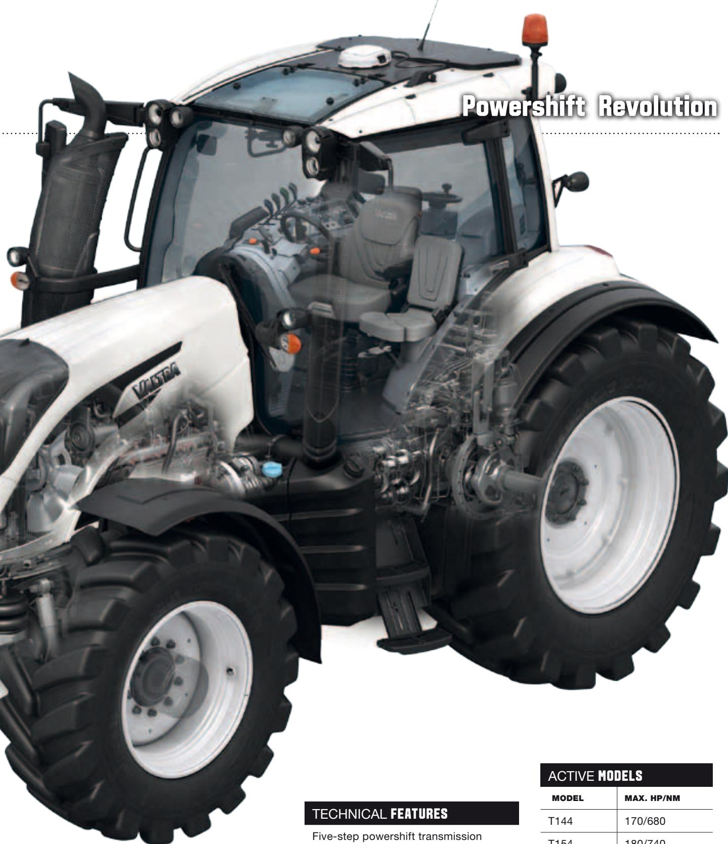
30 gears altogether. Both 40 and 50 km/h versions of the transmission are available. The Active transmission also features a useful hill hold function. •
