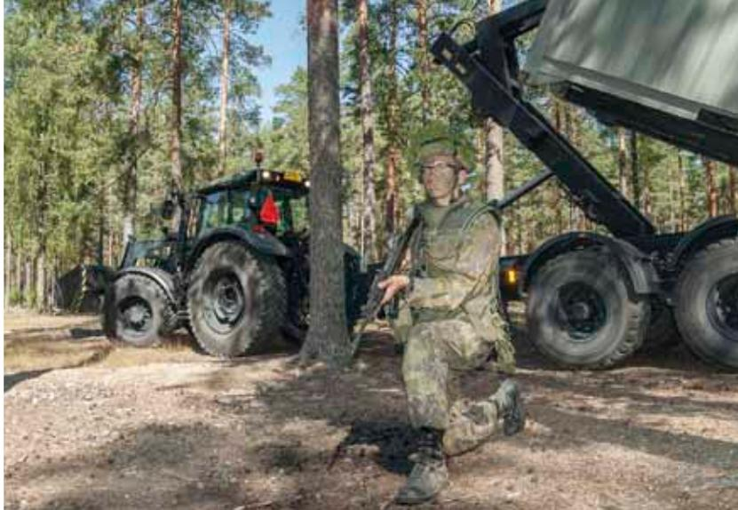
The tractors have already demonstrated their versatility with the Finnish Defence Forces. They can load and unload supplies in the forest, as well as pull containers weighing up to 16 tonnes and handle them with hook-lift trailers. In addition, tractors can be used to snow plough roads, clearing it for other vehicles.
