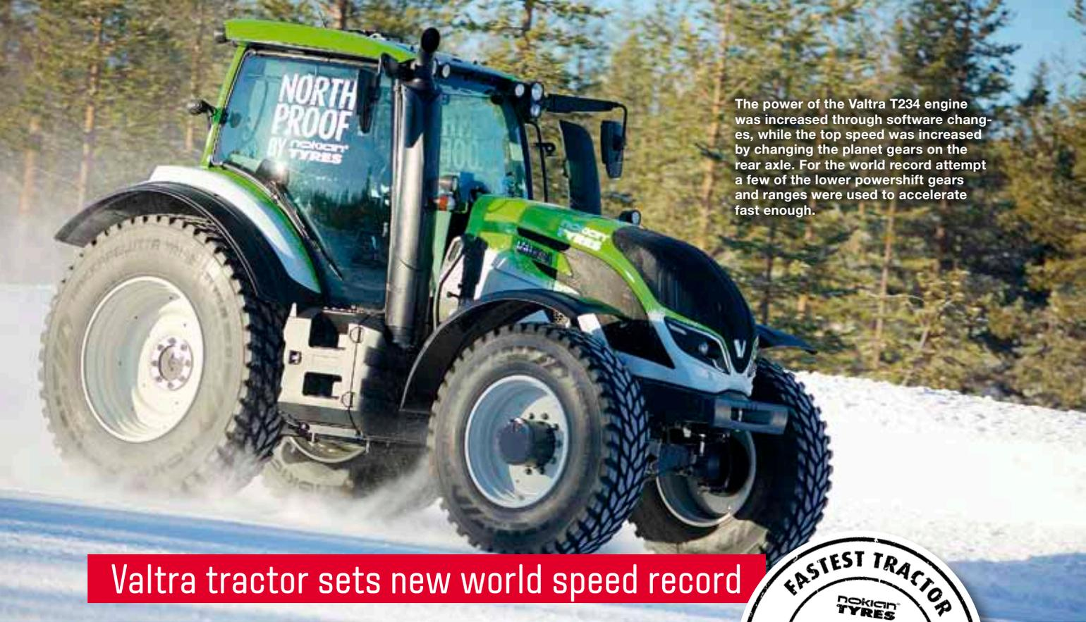
The power of the Valtra T234 engine was increased through software changes, while the top speed was increased by changing the planet gears on the rear axle. For the world record attempt a few of the lower powershift gears and ranges were used to accelerate fast enough.
