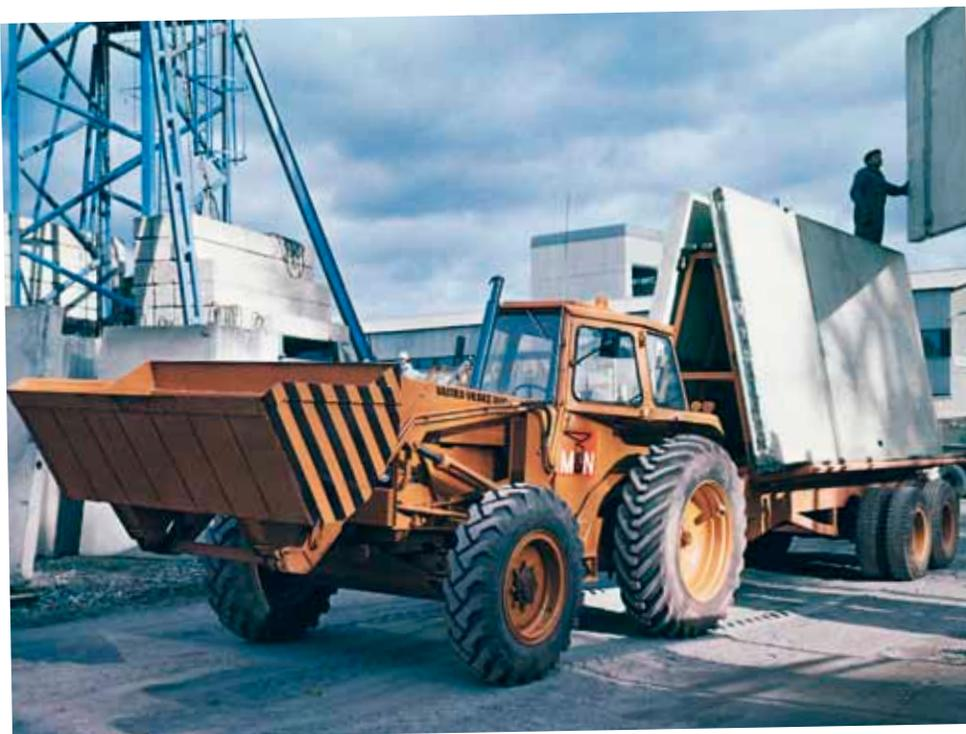
The Valmet 1100-4 was an extreme machine in 1969: 4WD, a four-cylinder turbo engine and 115 horsepower.
