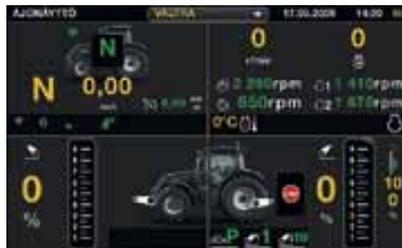
While driving all the required information can be displayed on its own screen or in four quadrants. The information displayed can be selected according to the task.
