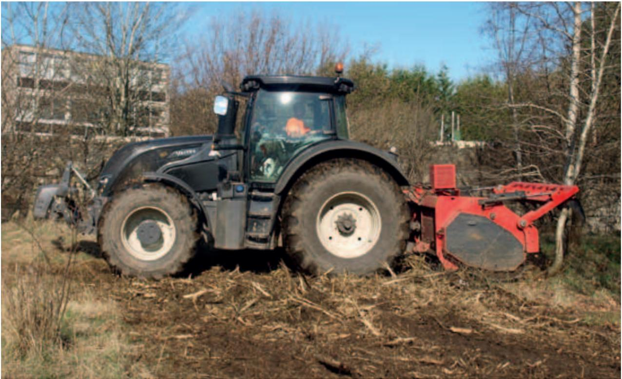
The Ahwi FM900 is one of the heaviest mulchers available. It is positive to handle – does not jump up and down – and managing it with the hydraulics on the S374 is simple.
