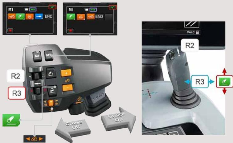
**1** Do you want to use the U-Pilot headland management system? Programming the system is easy. You can programme sequences according to time or distance. For example, when ploughing you can programme the M1 memory button to disengage the four-wheel-drive, cruise control and differential locks, raise the plough and turn – all with a single click of the button – when you get to the headland. Similarly, you can programme the M2 memory button to do the same in reverse
