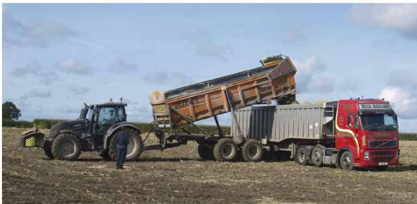
A full Dezeure self levelling trailer load of maize is transferred to the road truck. Control of the unloading is remote allowing the tractor driver to act as banksman for the truck driver.
