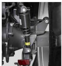
The mechanical cab suspension is adjustable and uses double Panhard rods to stabilise the cab.
