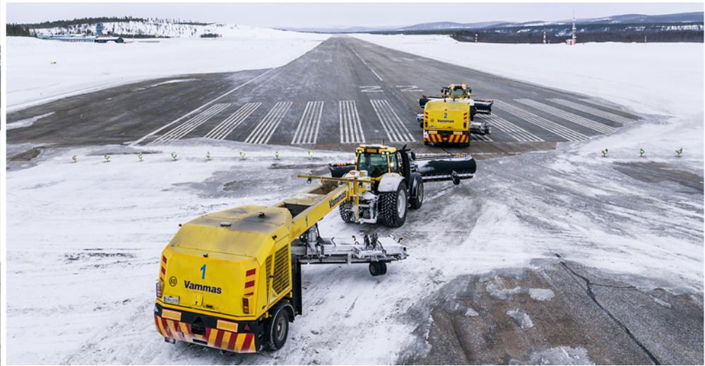
Valtra Guide automated steering is a big help when ploughing runways, also with a driver. The system identifies the edges and centre of the runway, even if it is completely covered in snow. GPS-based section control can further make sure that just the correct amount of de-icing chemicals are applied, which reduces impact on the environment as well as on running costs.
