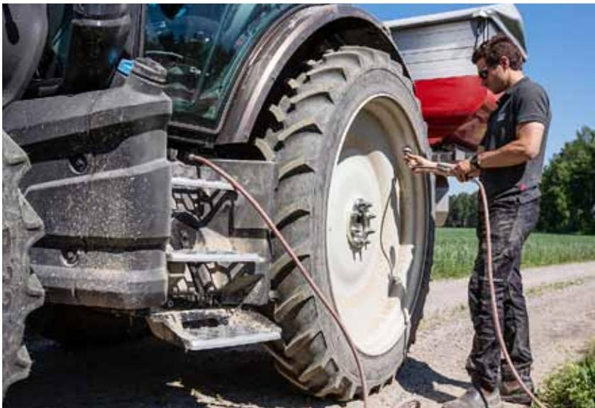
The new G Series is available with a compressed air connector on the side of the tractor by the cab steps, making it easy to adjust tyre pressures, for example.
