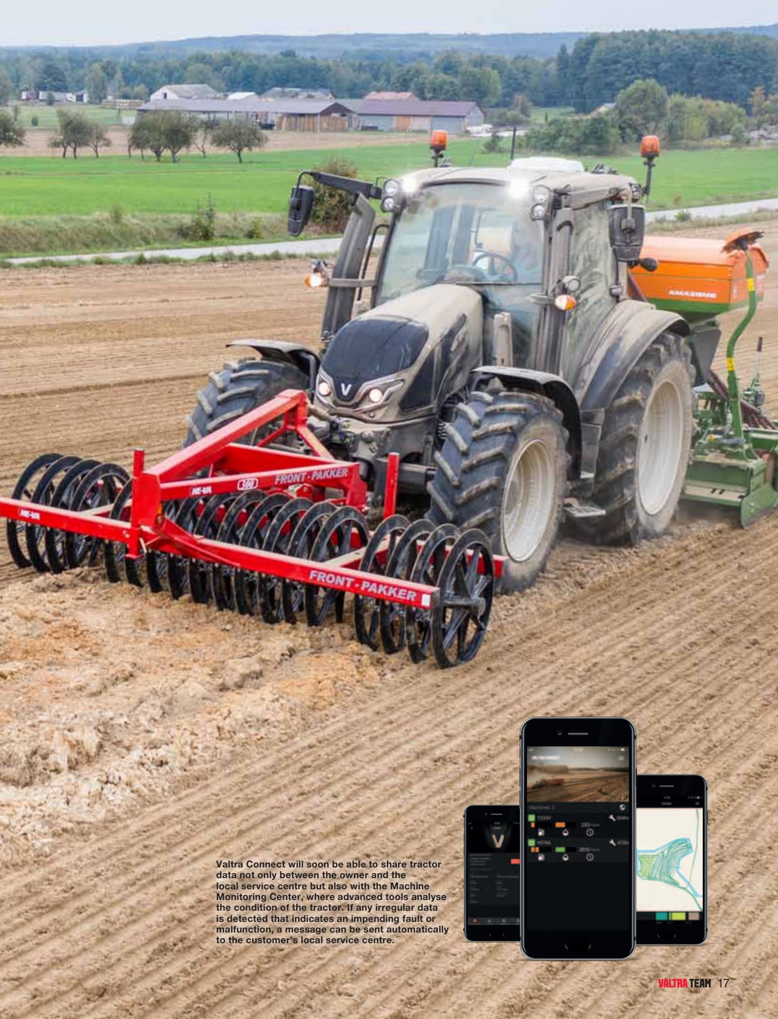
Valtra Connect will soon be able to share tractor data not only between the owner and the local service centre but also with the Machine Monitoring Center, where advanced tools analyse the condition of the tractor. If any irregular data is detected that indicates an impending fault or malfunction, a message can be sent automatically to the customer's local service centre.
