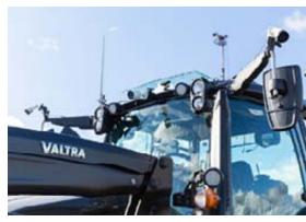
Cameras mounted on the outside show the operator what is happening around the tractor.
