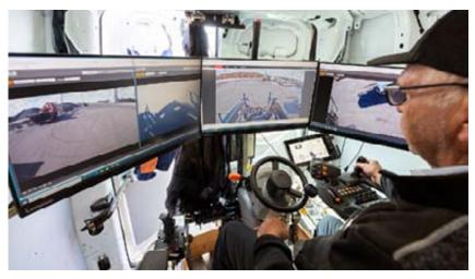
The tractor controls here are situated in a van. It is also possible to control a tractor remotely using the controls in another tractor or with more limitations using a portable control unit.
